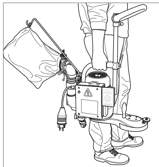
Fig. 53: The UNICO can be easily carried by being picked up by the pipe bend.
