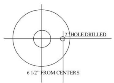
The hole in most buffers is drilled 6-1/2" from the center of the gearbox to the center of the hole. Due to the angled pipe on the UFO, some taller buffers may need the hole farther out.
