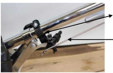
Drop the buffer handle to the lowest position that you would ever operate it. Mount the valve just above the buffer handle latch. The valve should be on the bottom side of the handle.
