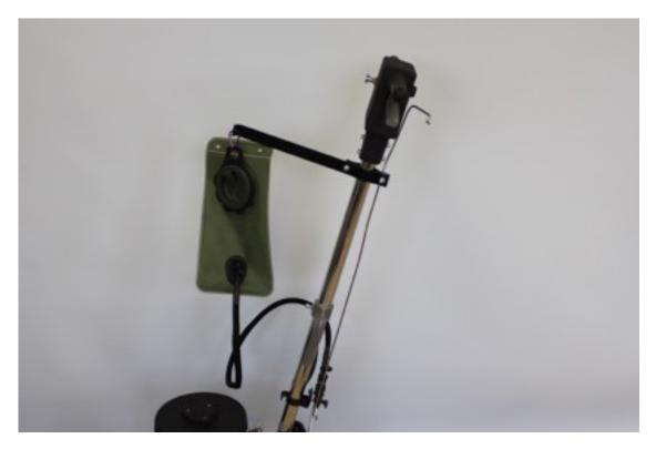
Hang the bag on the bracket and hook up the hose to the valve. ( Has push on locking fittings). The Hose valve should be on the control valve. Fill the Bag with stain and operate.
