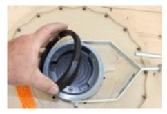
Remove plastic down feed hose. Remove Lock ring by turning COUNTER CLOCKWISE.
