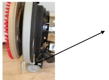
Install coater on buffer. Adjust the anchors so the vertical anchor contacts the left side of the buffer. The top anchor holds the main anchor just below the bottom lip of the buffer. It should allow the main anchor rod to float between the buffer frame and the rotating pad driver.
