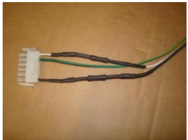
Photo 6 Shrink insulation to protect wires
