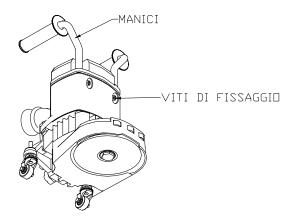
Loosen the screws that are fixing the motor cover and remove it.
