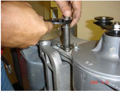
Fig. 5 Using a 1/4-20 bolt threaded into the shaft will prevent damage to the shaft surface when removing the shaft
