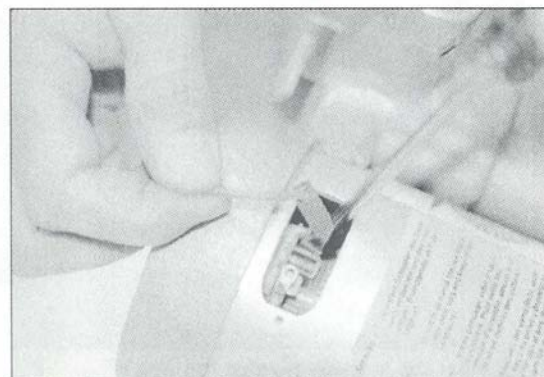
Fig. 32 With the tension clamp being held back, insert and connect the new carbon brushes.
