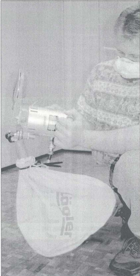
Fig. 18 Before emptying, shake the dust residue into the dust bag.
