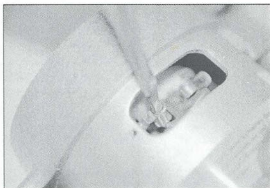
Fig. 30 ... and then, without letting any parts fall into the motor, loosen the clamping screws, before ...
