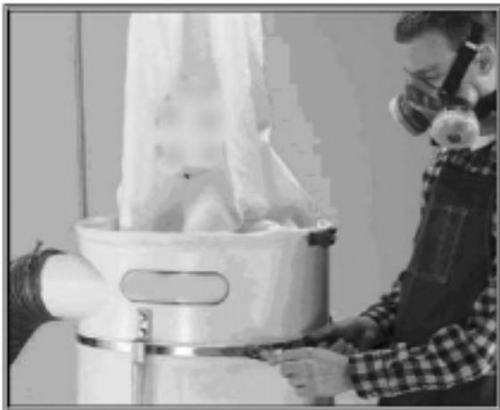
Figure 2. Wear a respirator when changing bags.
