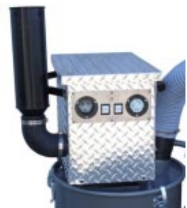
Photo 5 Install the exhaust muffler
