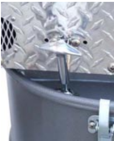
Photo 3 Latch the cabinet down with the spring latches
