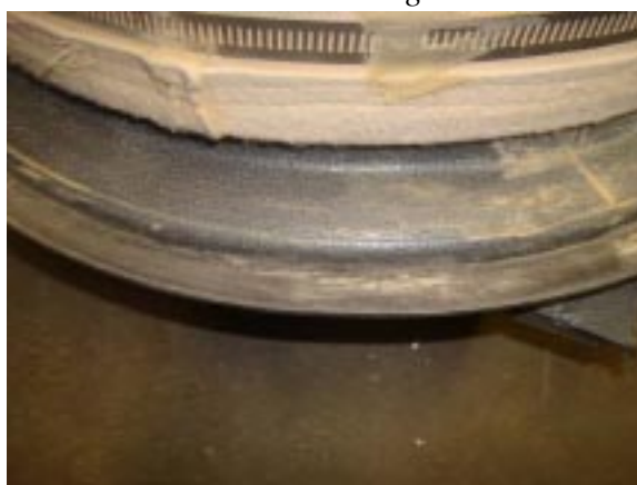
Photo 34 Inspect gasket for damage
