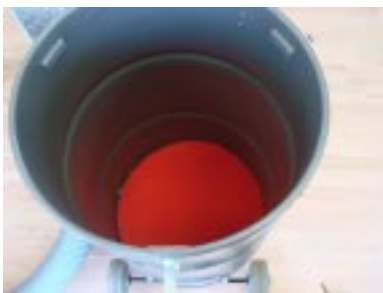
Photo 9 Place mesh pad in barrel
