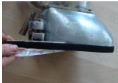
Photo 22 Install dust skirt
