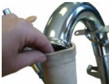
Photo 16 Stretch 2.5" connector over pipe
