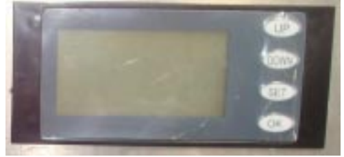
Photo 8 Combination power & hour meter
