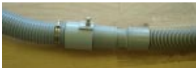
Photo 15 2" hose connected to 2.5" hose
